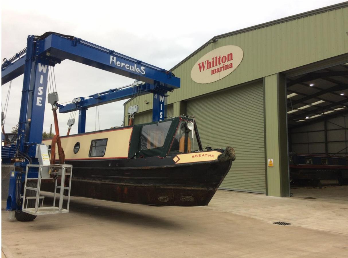
The boat lifting crane is probably the first purpose built facility of this kind on the UK inland waterways system. It will reduce our carbon footprint as a company because there will no longer be a necessity to have cranes travelling to and from our site for the purpose of lifting boats out of the water.
