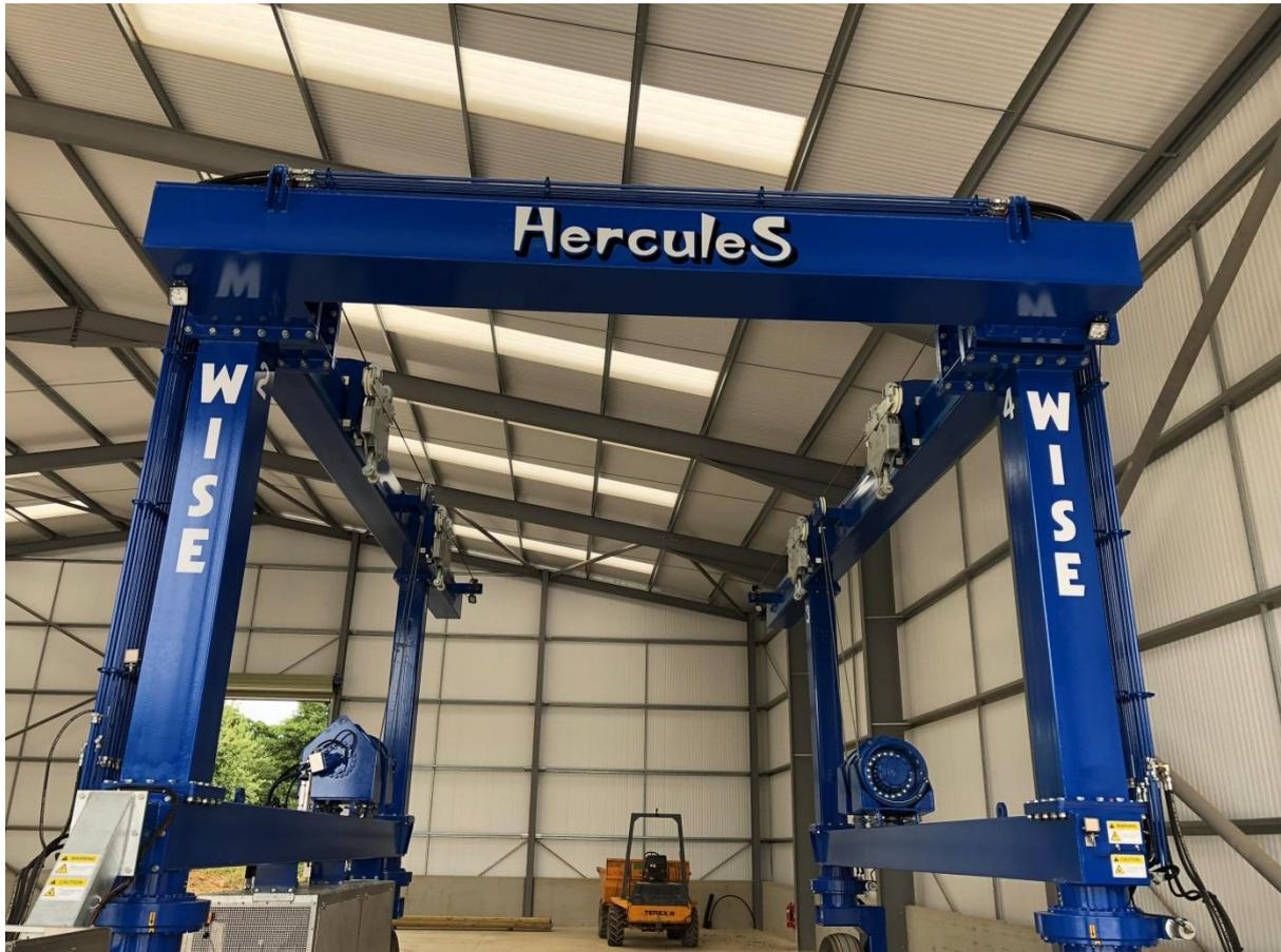
A new wharf has also been constructed to allow the Wise Hoist to manoeuvre over the water and lift out narrowboats when surveys are required. This will enable us to react a lot more quickly to our demands on site, which will speed up the boat sales process.
